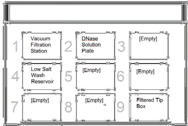
Figure 3. Bravo layout for DNase treatment step
