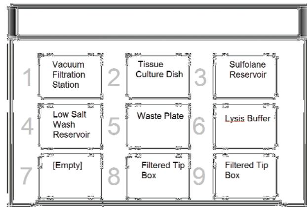
Figure 2. Bravo layout for lysis and binding steps
